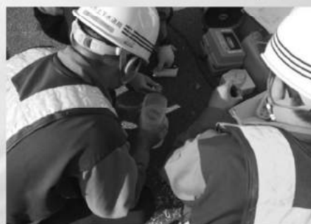
Check of water quality : residual chlorine
