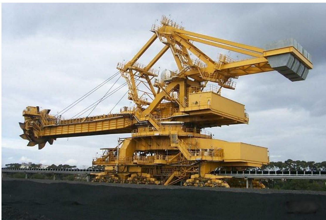
圖41 PWCS斗輪式堆/取煤機(Bucket Wheel Stacker/Reclaimer)
