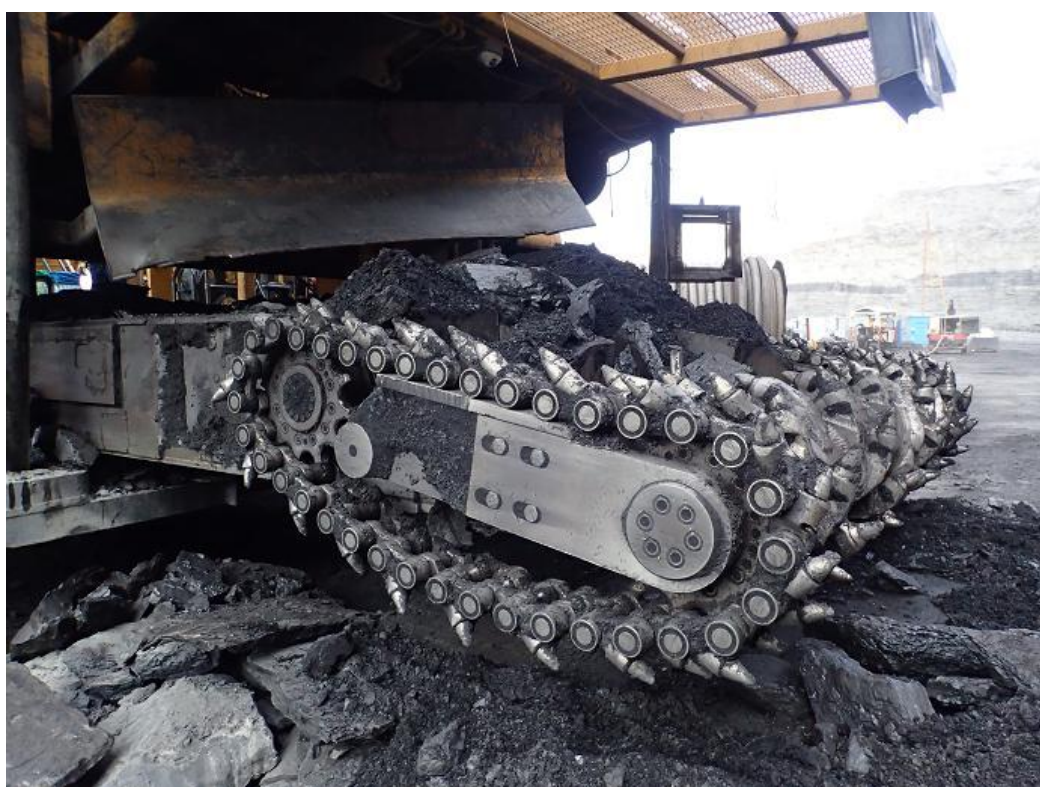
圖64 Drummond礦區Mina Pribbenow礦坑之High Wall Miner
