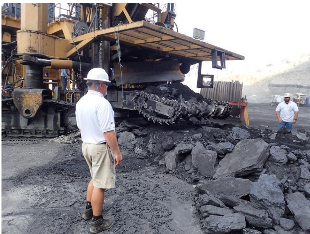
圖63 Drummond礦區Mina Pribbenow礦坑之High Wall Miner
