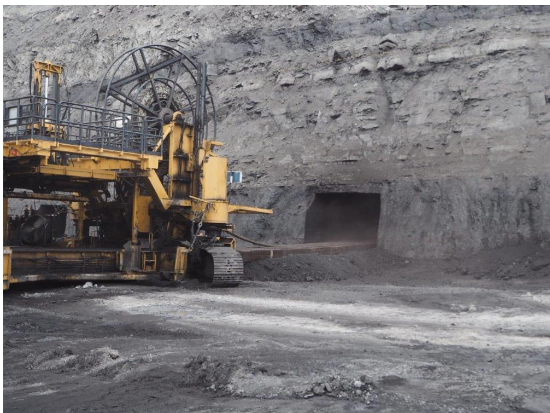
圖62 Drummond礦區Mina Pribbenow礦坑之High Wall Mining
