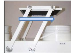
While the flat cover closing, Sensor positioning sheet will synchronously rotate with it until be detected by Flat cover closing positioning sensor with lighting on. Then flat cover will stop. "Cover close" on controller monitor will light on
