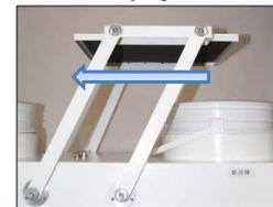
While the flat cover opening, Sensor positioning sheet will synchronously rotate with it until be detected by Flat cover opening positioning sensor with lighting on. Then flat cover will stop. “Cover open” on controller monitor will light on.
