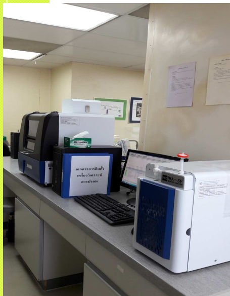
Atmospheric Hg analyzer (dual gold amalgam CVAFS)
