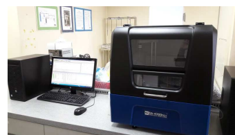
wet Hg deposition analyzer (gold amalgam CVAFS)
