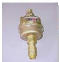
15 mm meter (Replace every 15 yrs or > 4,000 m 3 )
