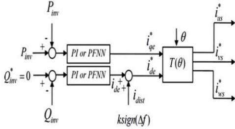
Fig. 2 Control block of proposed islanding detection method
