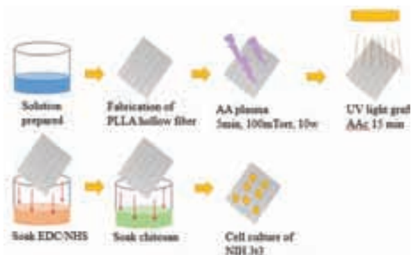
Fig. 2 Schematic reaction steps for the immobilization of chitosan on MTAMs by plasma and grafting treatments are shown
