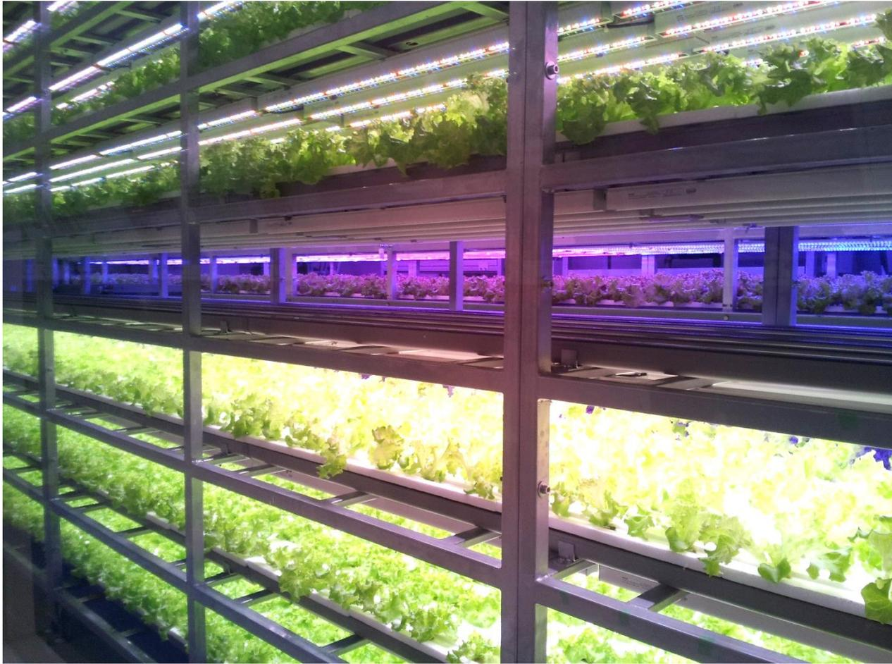
A CPPS (closed plant production system) for production of transplants with a floor area of 16 m<sup>2</sup>. In 2014, about 300 units of CPPS are in use at 130 different locations in Japan.
