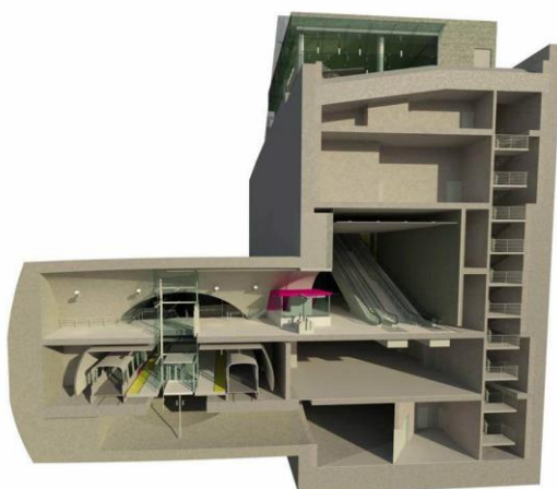
車站橫向斷面 (CTS section through Washington, 2012-10-11)
