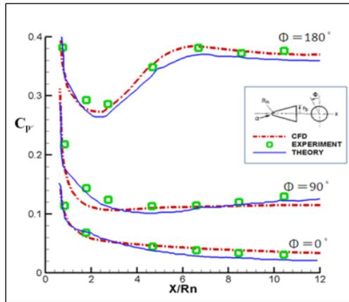
Fig. 5. Comparison the  $C_p$  values of computation with the experimental and theory of Rakich and Cleary.
