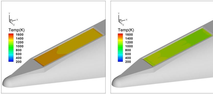
Fig. 11. 20km, 60sec, optical window Temp. in adiabatic, heat flux condition.
