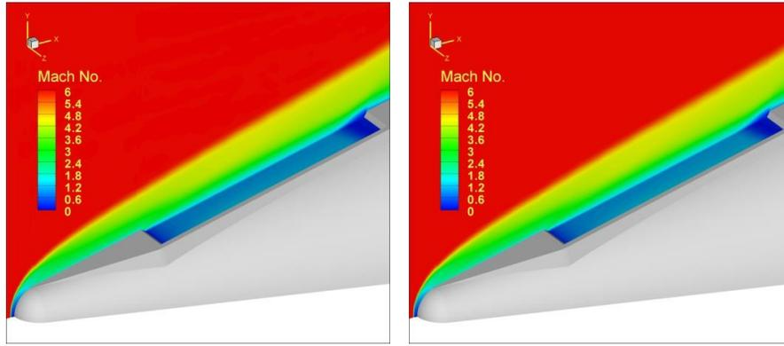
Fig. 9. 20km, 60sec, Mach No. contour in adiabatic, heat flux condition respectively.
