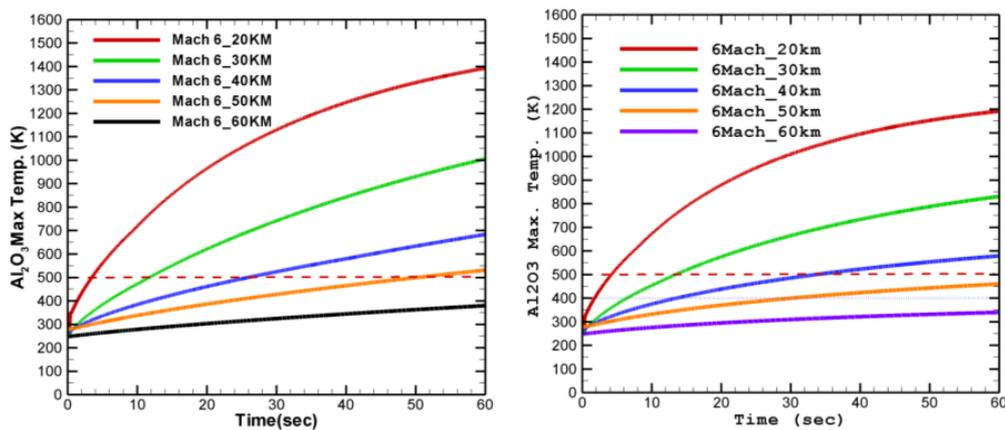
Fig.14. 20~60km, optical window  $T_{max}$ -Time in adiabatic, heat flux condition.
