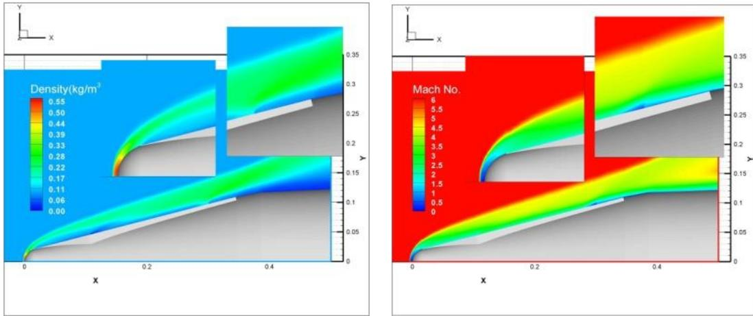
Fig. 6. Pressure, density and Mach number contour respectively.
