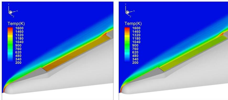
Fig. 10. 20km, 60sec, Temp. contour in adiabatic, heat flux condition respectively.
