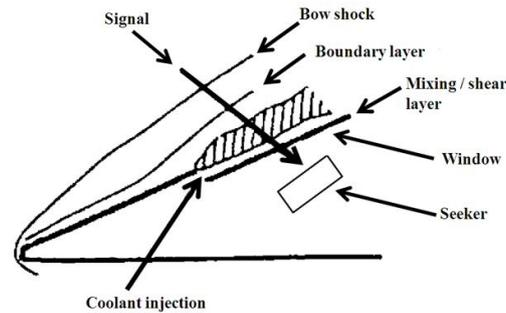
Fig. 1. Schematic diagram of aero-optical effects [1]
