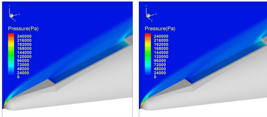
Fig. 7. 20km, 60sec, pressure contour in adiabatic, heat flux condition respectively.
