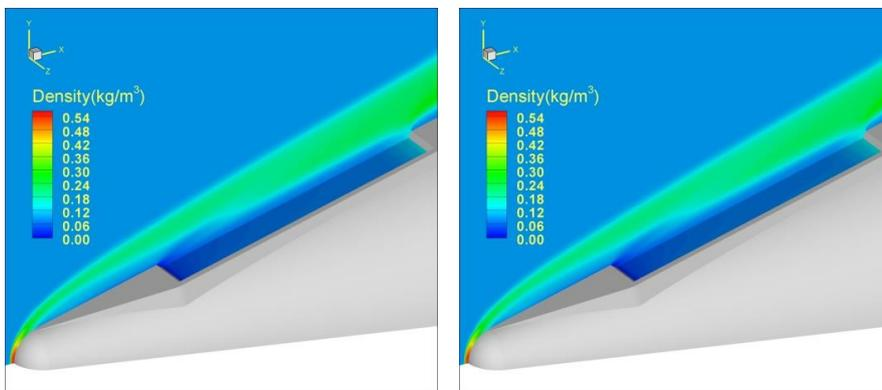
Fig. 8. 20km, 60sec, density contour in adiabatic, heat flux condition respectively.
