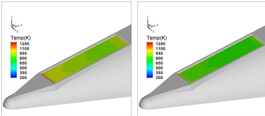
Fig. 12. 30km, 60sec, optical window Temp. in adiabatic, heat flux condition.
