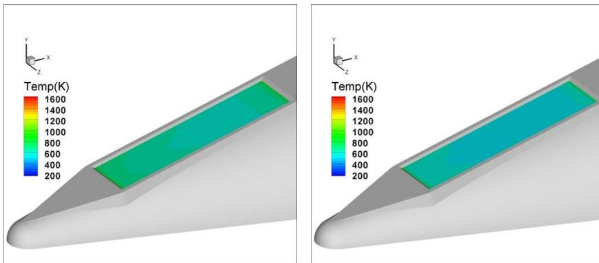
Fig. 13. 40km, 60sec, optical window Temp. in adiabatic, heat flux condition.
