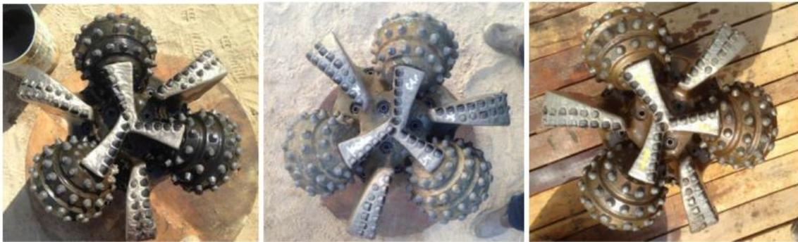
Figure 13—22 inch Hybrid dull grading pictures for Well 5, 6 and 7
