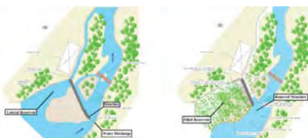
Figure 2: Planned removal of Aval Rabaud weir.
