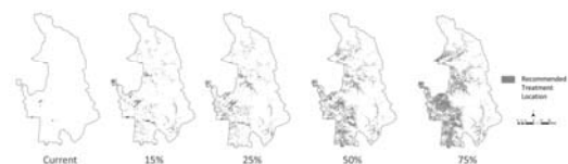
Figure 2: Each panel shows recommended treatment alternatives arrived at by maximizing ROI. Moving right across the panels shows increased treatment budgets.
