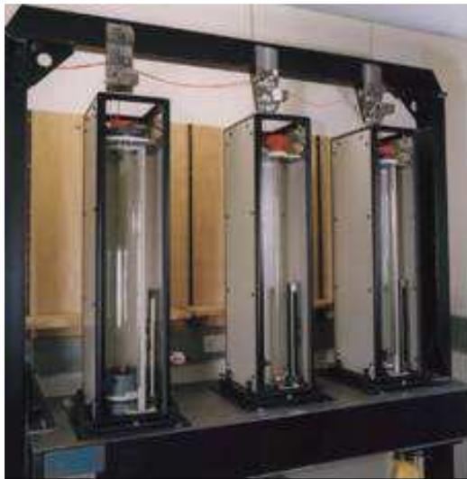
圖 24、Interferometric piston prover system at PTB
