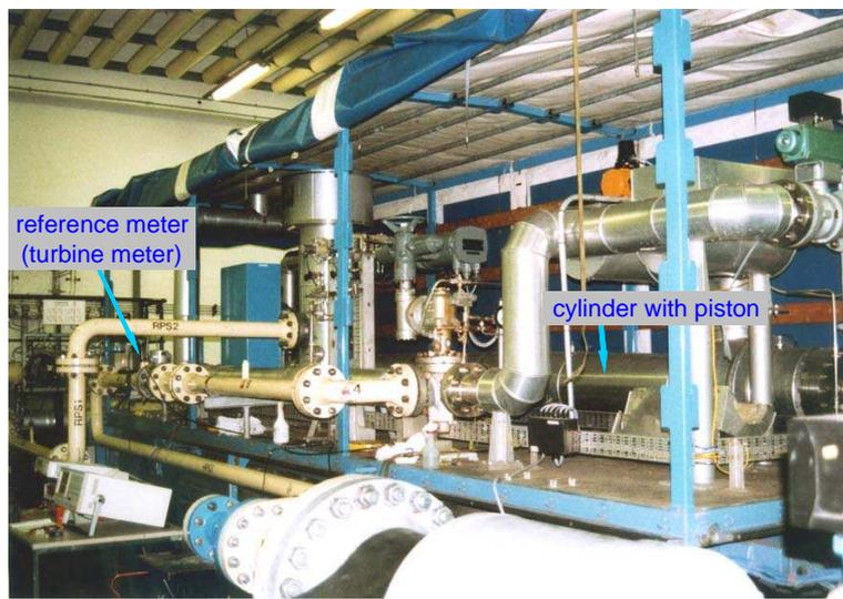
圖 18、high pressure piston prover (HPPP) with reference
