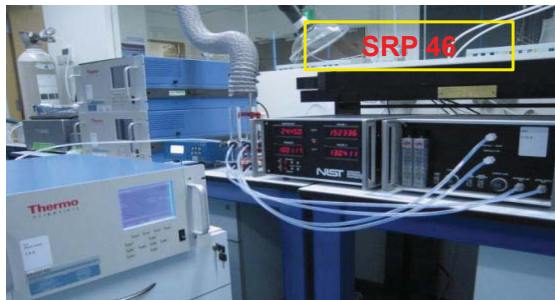
NMC ozone analyzer calibration facility
