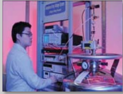
Josephson array voltage primary standard
