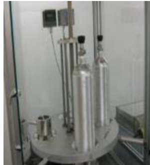
Weighing of cylinder with gas standards
