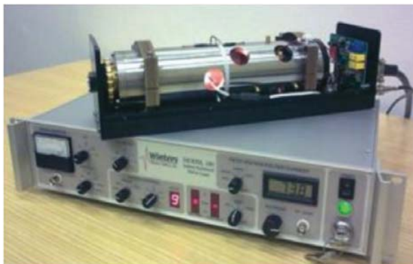
Primary realisation of the metre using iodine-stabilised He-Ne laser with wavelength of 633 nm
