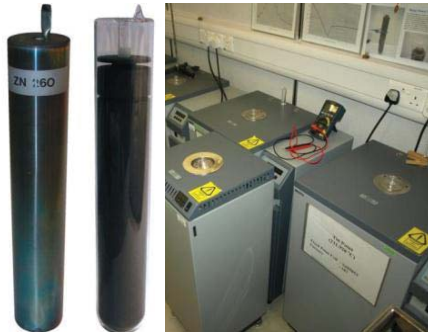
Fixed points for realisation of ITS-90 from -189.3442\text{ }^{\circ}\text{C} to 961.78\text{ }^{\circ}\text{C}
