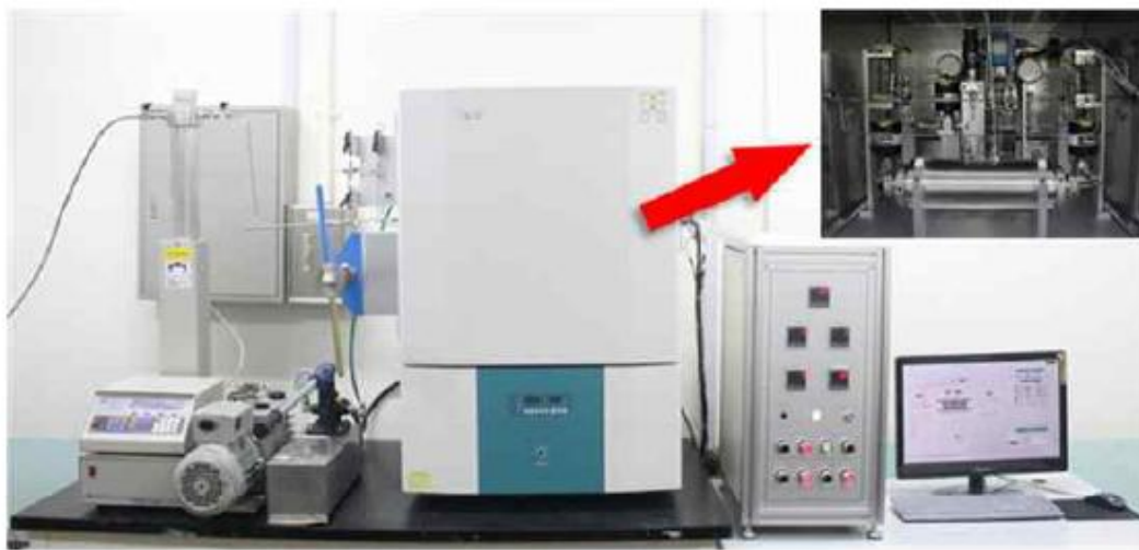
圖 3.21 Low permeability measurement apparatus
