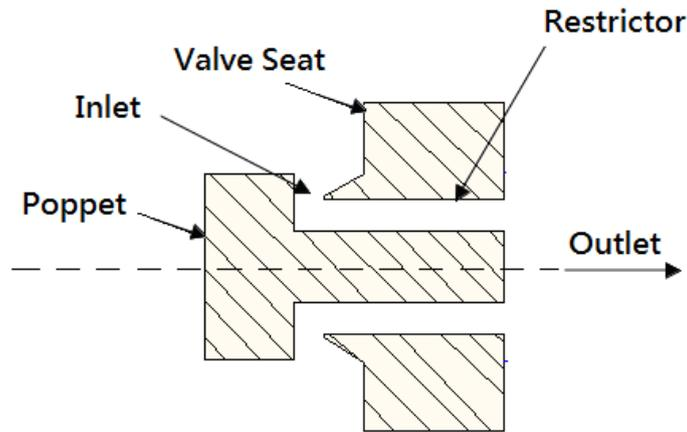
Fig. 2: The geometry of the main metering restrictor
