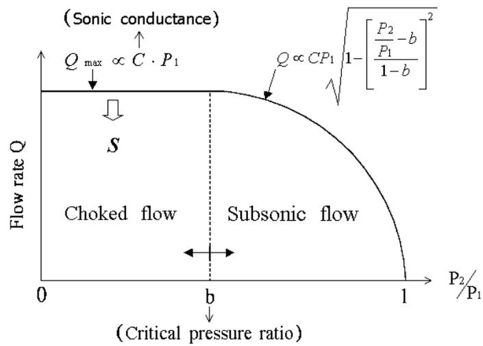
Fig. 3: The typical airflow property through a pneumatic flow restrictor
