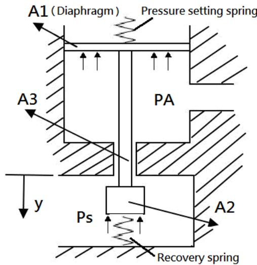
Fig. 7 : Scheme of the poppet and valve body geometry
