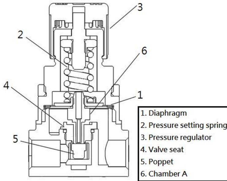
Fig. 1: The chosen pneumatic pressure regulator
