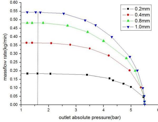
Fig. 6: Mass flow-rate characteristic curves for the main metering restrictor
