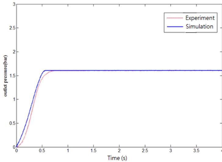
Fig. 10: *Simulation and experimental dynamic pressure response for 1.6 bar output pressure control*
