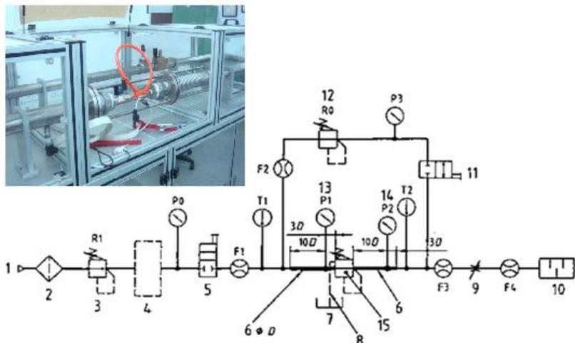
Fig. 12: Real test bench for the pneumatic pressure regulator according to ISO 6953 standard
