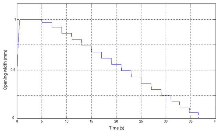
Fig. 11: *Stepwise variable input signal of opening width for the continuous measurement of the P/Q char. curves*
