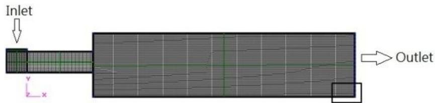
Fig. 4 : Two-dimensional Cartesian coordinate mesh model of the flow field (Opening width= 1.0mm)
