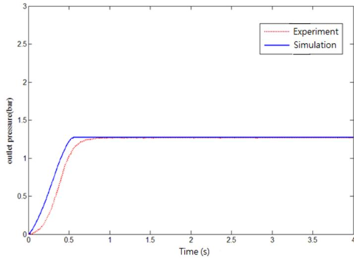
Fig. 9: *Simulation and experimental dynamic pressure response for 1.25 bar output pressure control*
