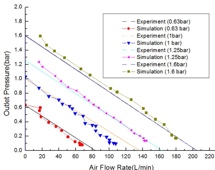
Fig. 13 : Comparisons between the experimental and simulation P/Q characteristic family curves
