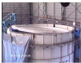
Batteries used for Fire Experiment 480 cells of the 18350 type cell (= 95 battery packs of video and other DIY tool) in a plastic container
