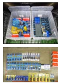
Batteries used for Fire Experiment 480 cells of the 18350 type cell (= 95 battery packs of video and other DIY tool) in a plastic container
