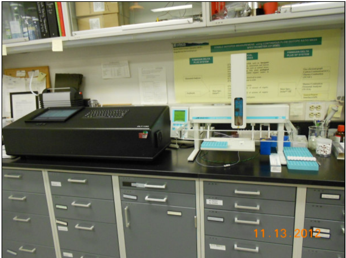
Liquid-water Isotope Analyzer (DLT-100) for \delta^2\text{H} and \delta^{18}\text{O}
