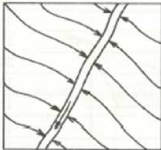
Natural water channel or grass waterway
