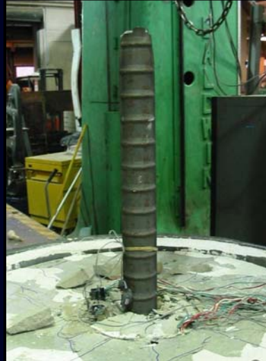
Long l_e : bar fracture, embedment of 16 d_b
