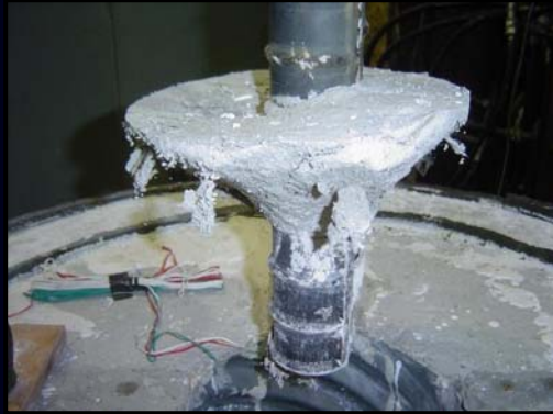
Short l_e : pullout failure
