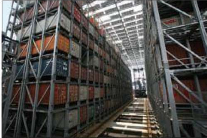
Interior and exterior views of the high density container racks developed by JFE Engineering for NYK Line at Ohi Pier, Tokyo
