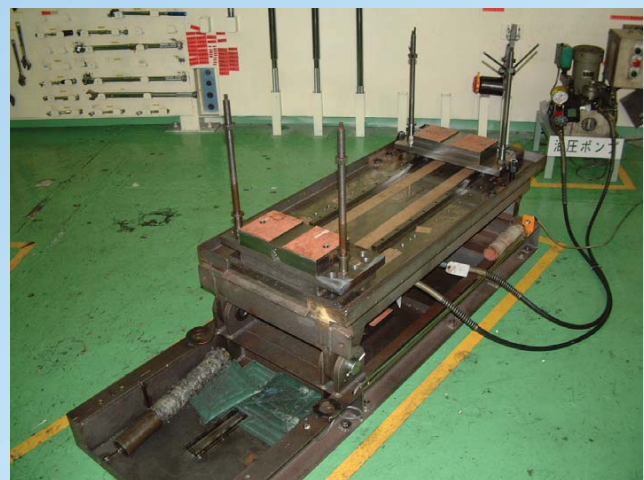
For tightening of bolts/nuts of the hydraulic cylinder with torque
