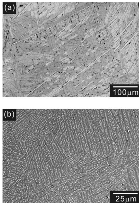
Figure 1 Images of as-cast Ti-7Cu alloys: (a) OM, (b) SEM-BSE.
