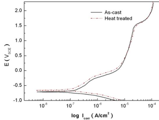
Figure 4 Experimental potentiodynamic anodic polarization curves for Ti-7Cu alloys samples in a 0.9 wt.% NaCl solution at 25 °C.
