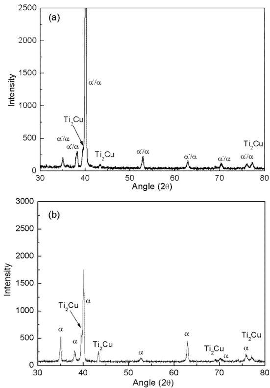
Figure 3 X-ray diffraction patterns of: (a) as-cast sample and (b) heat treated sample.
