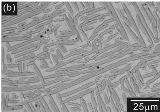
Figure 2 Images of heat-treatment Ti-7Cu alloys: (a) OM, (b) SEM-BSE.
