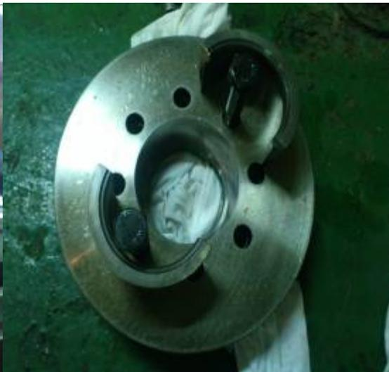
Piston with Ridged Valve Cone Piece
