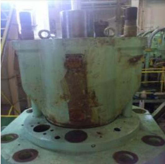
Exhaust Valve of Cylinder Head
