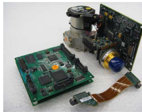
VE1.6 with detector, cooler, and ADC.
