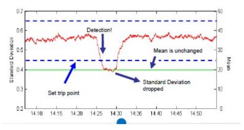
圖-10 SPM Detects Plugged Impulse Line
