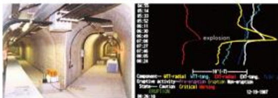
The tilt and strain observation in an underground tunnel, and tilt and strain records associated with an explosive eruption.
