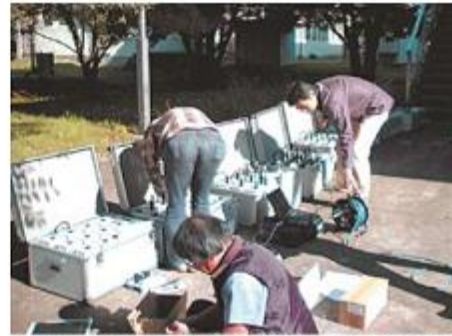
Preparing mobile seismic recorders for a temporal seismic observation
