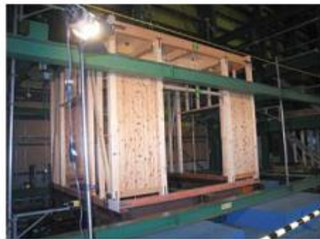
Shaking table test of a newly proposed column-wall
