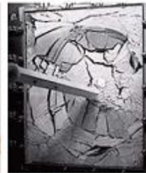
Impact test to glass by flying debris
