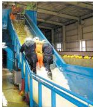
Evacuation experiment through stairs in case of underground inundation
