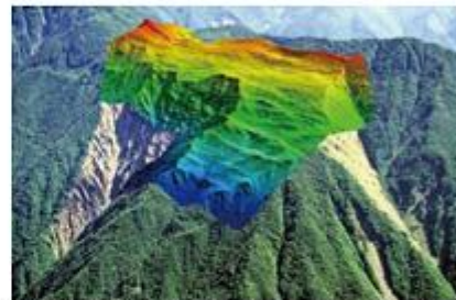
Gravitational slope deformation in the Akaishi Mountains. Numerous number of linear depressions were identified by using the high-resolution DEM obtained by the air-borne laser scanner.
