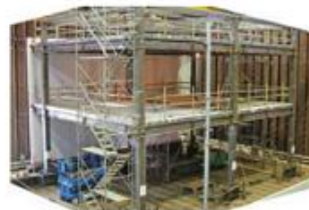
Collapse experiment of actual-size steel structure
