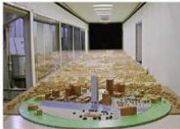
Wind tunnel test for wind pressure and velocity around tall buildings.
