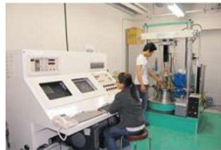
Ring shear apparatus for simulating landslides triggered by earthquakes and heavy rainfalls
