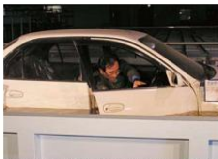
Real-scale experiment apparatus of the evacuation from a submerged car
