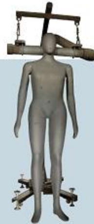
防火服の耐熱性能評価に用いるサーマルマネキン A thermal mannequin used to assess the heat resistance performance of protective clothing
