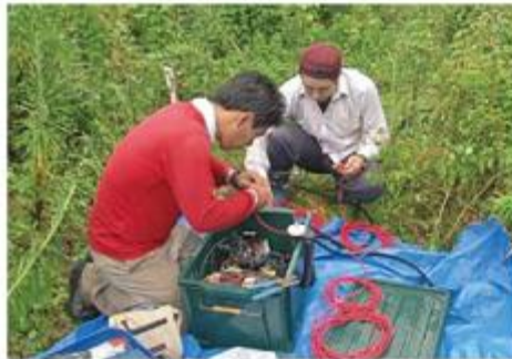
Set up an electromagnetic survey system
