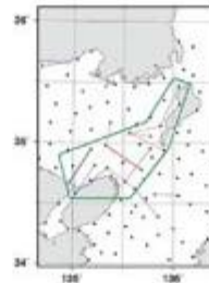
Deceleration of strain rate in the Kinki district (Red line indicates contracted baseline and blue line indicates extended line)
