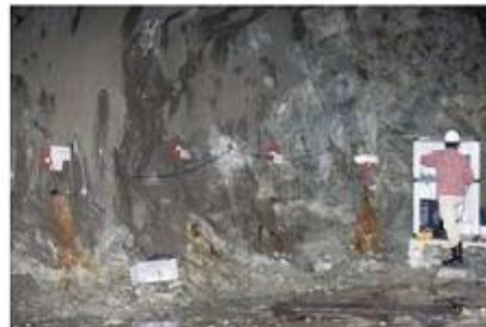
Pore pressure monitoring of borehole at the Kamioka mine
