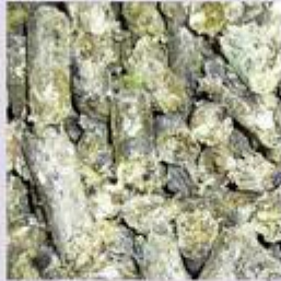
RDF-5 (可燃廃棄物を粉碎し圧縮して成形したもの) RDF-5 (created by crushing flammable refuse and then pressure forming it)
