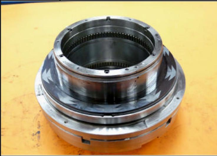
Picture 10 shows the outboard mating ring assembly.
