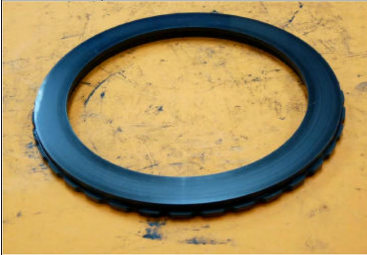
Picture 5 shows the inboard primary ring.
