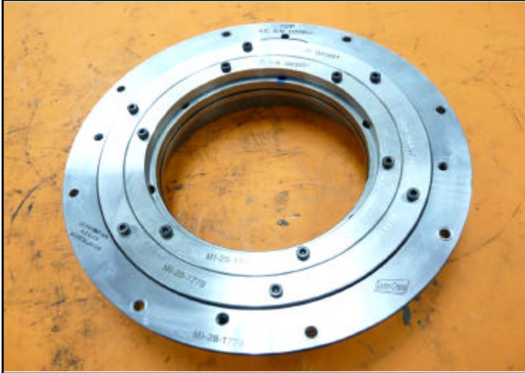
Picture 19 shows the T82 barrier seal.
