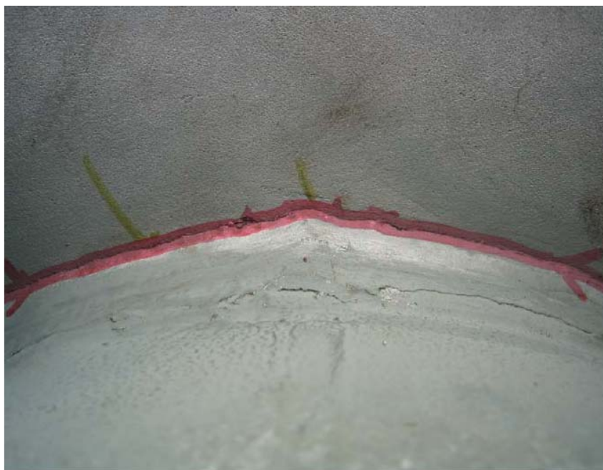
Figure 2.5 Fatigue Crack at End Plate Weld Toe in Laboratory Specimen
