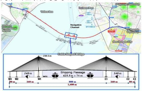
圖 2.3 斜張橋(Cable-stayed Bridge, 1/2)
