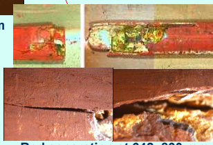
Rod separation at 642-830 mm
