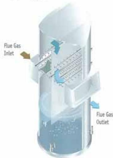
Return flow type was developed as an alternative to the conventional absorber. The SO<sub>2</sub> removal efficiency is higher than that of a conventional vertical absorber.
