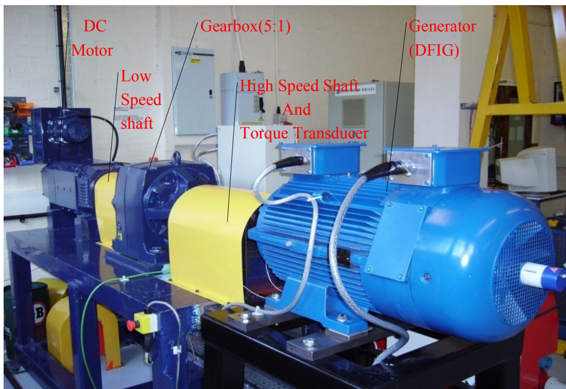
圖 3.2 A photograph of the Test Rig
