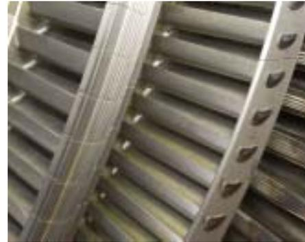
Integral Cover Buckets      Buckets with Peened-on Cover
