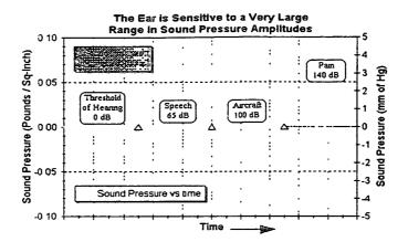
In the final figure, the vertical scale is magnified yet another 100 times (10,000 times the second figure) and the speech at 65 dB is now just perceptible. To complete the picture, the smallest sound a healthy human can detect is near 0 decibels. For that sound pressure to be perceptible on this type of graph, the vertical scale would have to be magnified another 1,000 times over that shown in the final figure.
