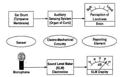
There are three important components to both systems. The first is the sound pressure sensing element, the eardrum (tympanic membrane) in the human system, and the thin microphone diaphragm in the sound level meter. Both are held tightly in place, and both vibrate by minute amounts as sound pressure impinges on them.
