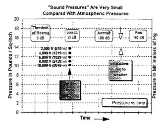
At the pressure scale shown in the second figure, only the 140 decibel sound pressure fluctuations are visible, an indication of just how small even loud sound pressure fluctuations really are. These pressure differences about atmospheric pressure are referred to as sound pressure. Sound pressures are measured as if the ambient atmospheric pressure were the zero line, with pressures above atmospheric considered positive, and pressures below atmospheric, negative.
