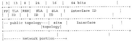
The public routing topology is represented by a /48, giving each site 16 bits to create their local topology. The host portion is represented by the last 64 bits of the address.
